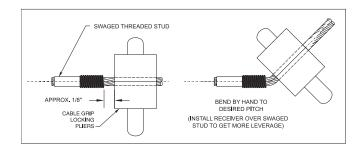
3. Install the Receiver in the post at the bottom of the stairway, following the instructions in the "Installing Cable" section for installing Invisiware Receiver at Post A. Make sure the stud is flush with the outside wall of the post. See illustration at right.
