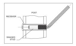
**4. Pull the cable** to the hole in the post at the top of the stairway where the Receiver will be installed on the other end of the cable. Mark the cable at the center point of the hole. See illustration at right.
