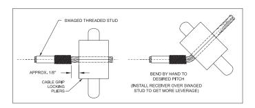
5. Install the Receiver in the post, following the instructions for installing Invisiware® Receivers at Post B in the "Installing Cable" on pages 4-9. When tensioned, the cables will self-align with the fitting at the other end of the cable run.
