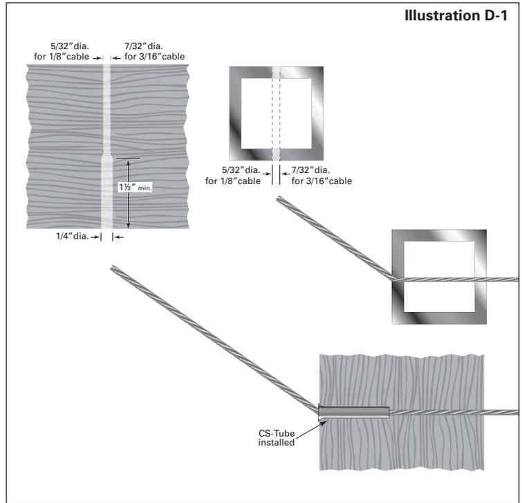
1. For wood posts only, insert a Post Protector Tube (order separately from Accessories) into all wood posts where the cable angles out of the post. Drill 1/4" diameter holes 1-1/2" deep into the face of the post where each cable angles out of the post. Force tube into post so it is flush with post face. (Illustration D-1)
