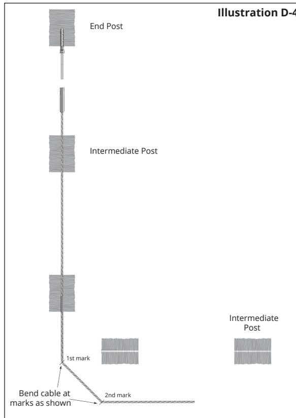
6. Bend the cable in both locations that you have marked to approximately 45° (in the same plane). Use a tool such as Ultra-tec Cable Gripping Pliers to help you make “sharp” bends in your cables at the marked locations. (Illustration D-4)
