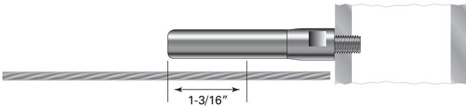
4. Push the cable into the hole in the fitting as far as it will go (approx. 1-1/16"). Twist the cable in a right hand direction as you push it into the fitting.
