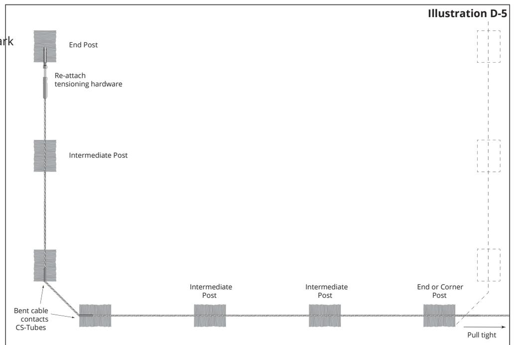
8. When the bare end of the cable has been passed through all remaining intermediate posts (if another 2-post corner is encountered, repeat Steps 1-7) proceed to Section E of the installation instructions for your kit application.
