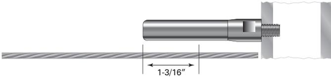
4. Push the cable into the hole in the fitting as far as it will go (approx. 1-1/16"). Twist the cable in a right hand direction as you push it into the fitting.
