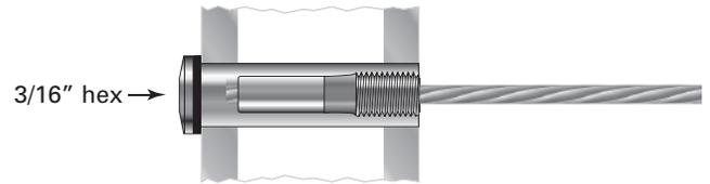
The swaging stud will be pulled into the Receiver by the tensioning.
