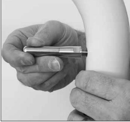
2. Thread the Push-Lock® coupler onto the post and tighten with 7/16" wrench.
