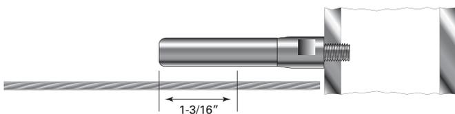
4. At opposite end post with tensioning terminal, detach the body from the Threaded Bolt to allow cable slack so you can perform the next step.
