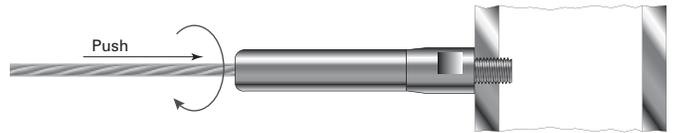
**Note:** If you have trouble inserting the cable into the fitting, it may be because the locking wedges have become stuck. This is not a defect! Here's what you can do to "free the wedges" —
