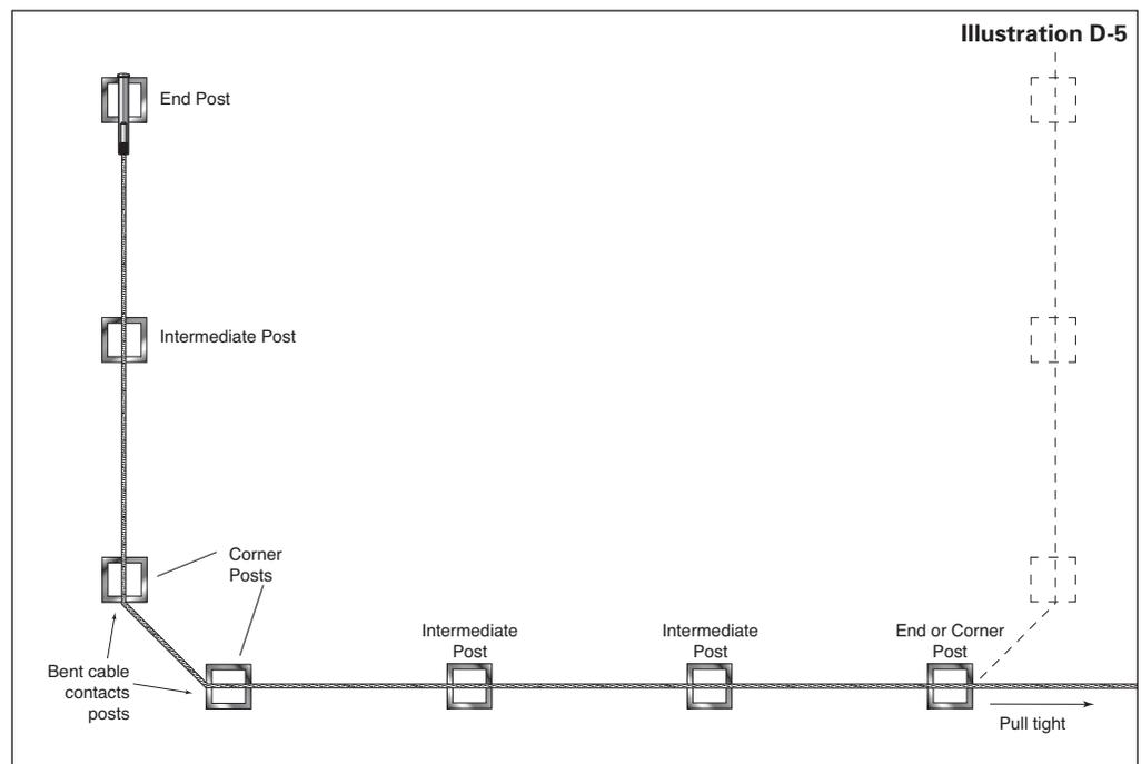
**5g.** When the bare end of the cable has been passed through all remaining intermediate posts (and maybe one more 2-post corner configuration) proceed to Step 6 of the installation instructions for your kit application.
