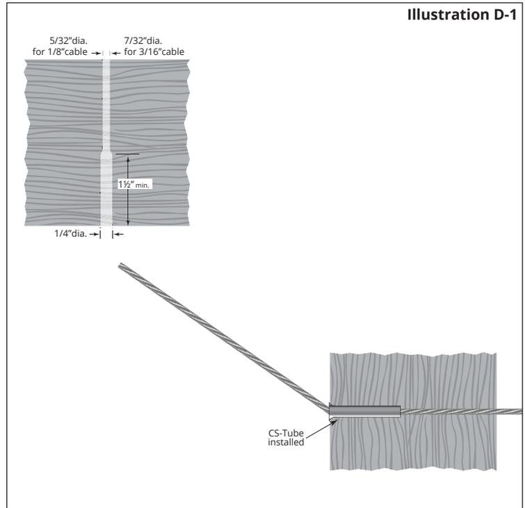
2. As you feed the bare end of your cable through your intermediate posts (per Section C in your installation instructions), stop after you feed it through the first of your two corner posts.
