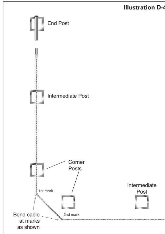
**5e.** Bend the cable in both locations that you have marked to approximately 45° (on the same plane). Use a tool such as Ultra-tec Cable Gripping Pliers to help you make “sharp” bends in your cables at the marked locations. (Illustration D-4)
